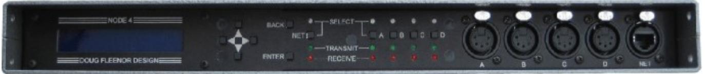
The Node 4 is an Ethernet to DMX interface. It accepts either Artistic License's ArtNet (version 3) or PLASA's streaming ACN (ANSI E1.31) protocol. There are four fully isolated DMX ports. Each port can be configured as either an input or as an output. All of the data connectors can be mounted on either the front or rear panel. Their location can be changed in the field to accommodate fixed or touring installations. Optional terminal block connections are available for the DMX ports.
