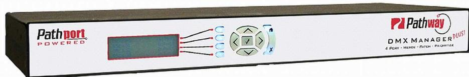
Each port has both a male and female connector with the unused connector available as a pass through. An integrated Ethernet switch allows multiple boxes to be chained together. The Manager Plus takes up one RU of space and ships with rack ears. The universal power supply accepts voltages between 85 and 240 VAC. The Manager Plus does not support Net2.
